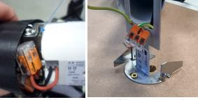
In 7.2.1 earthing contact shall be permanently and reliably connected to a protective earthing terminal or protective earthing
